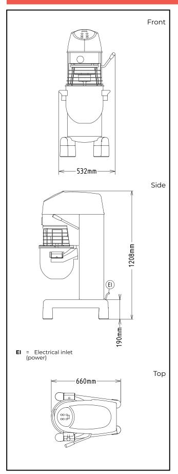
Electric Supply voltage: 200-240 V/1N ph/50/60 Hz **Electrical power max:** 1.1 kW **Total Watts:** 1.1 kW Capacity: Performance (up to): 7 kg/Cycle Capacity: 30 litres Key Information: External dimensions, Width: 532 mm External dimensions, 685 mm Depth: External dimensions, Height: 1208 mm **Shipping weight:** 111 kg **Cold water paste:** 7 kg with Spiral hook **Egg whites:** 50 with Whisk
